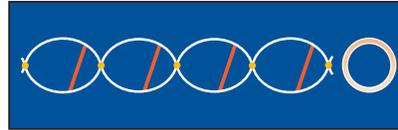
While in this deformed shape, the tubing is cooled. The crystals then reappear, thereby locking the structure together indefinitely in the expanded form. This is the form in which the material is supplied to customers.
