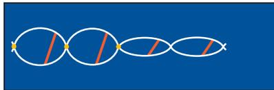
A user reheats the product, melting the crystals. The crosslinks allow the material to return to its original shape. This is the perfect elastic memory of crosslinked material.
