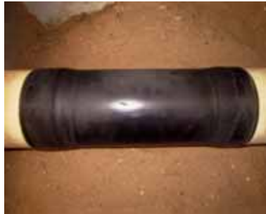
HTLP-PP after 100 cycles in soil stress test at 110°C (230°F) Covalence® 3-layer heat-shrinkable sleeves have excellent resistance to both cathodic disbondment and hot water immersion resistance, even at maximum operating temperature. They fully resist shear forces induced by soil and thermal movements.
